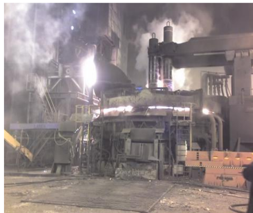
Figure 5.4 Image of operating electric arc furnace
